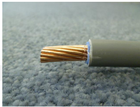
Example of 19 strand striped conductor
