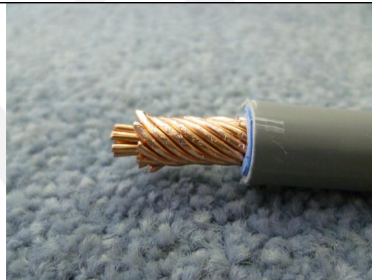
Example of twisted 19 strand conductor
