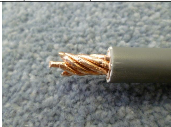
Example of twisted 7 strand conductor
